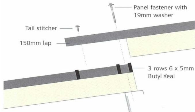
Figure 03: End lap fixing details - roof panels
