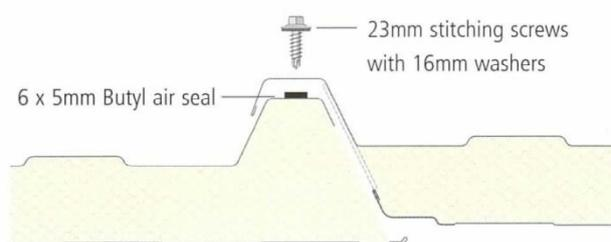
Where end laps are required on large span roofs or where rooflights are to be incorporated within the design of the roof. End laps are formed where the weather sheet of the upper panel overlaps the lower panel. The end lap dimension is governed by the building design and pitch of roof. These laps are sealed with **three** runs of Butyl Lap Strip 6mm wide x 5mm high. The first run is fixed 10 – 15mm
